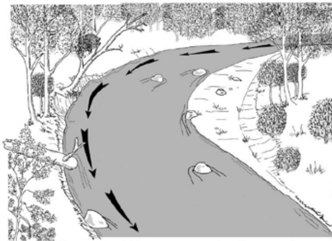
ACTIVE BANK SCOUR WITH VERTICAL CUT BANKS, SLUMP BLOCKS, AND FALLING VEGETATION
